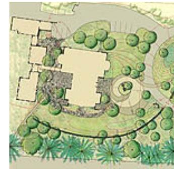
*Site plan showing the approach, field stone wall, and retention ponds.
